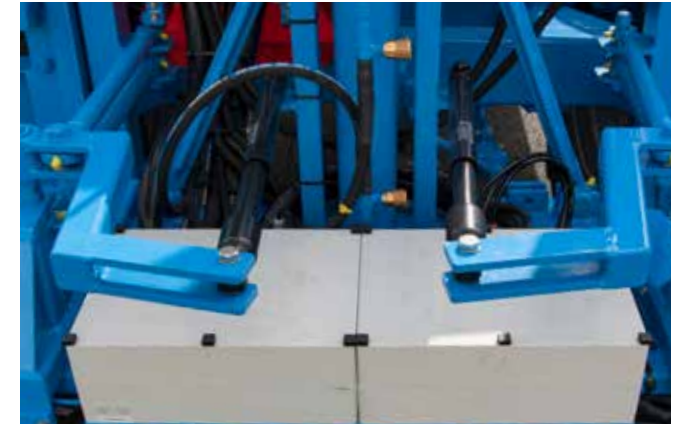
Oil shock absorbers slow boom movement in both ways.
