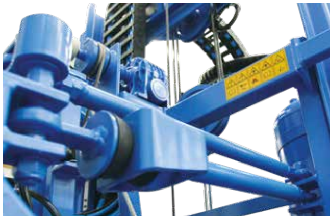
Stabilizers lower boom oscillation back and forth.
