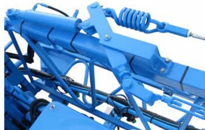
Detail of hydraulic boom folding to the back
