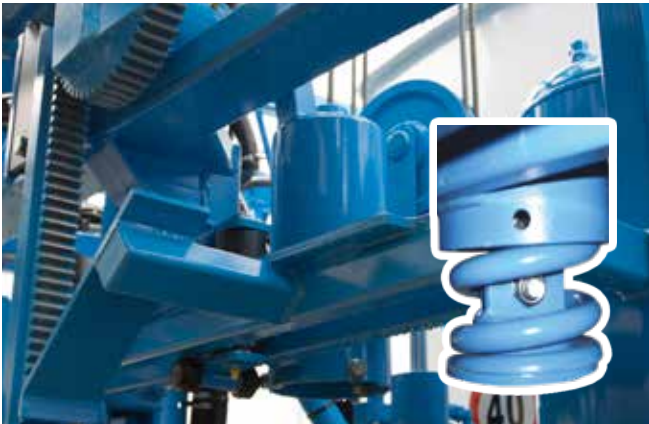
Soft vertical boom suspension is ensured by a coil spring.
