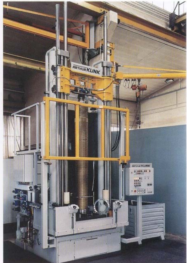
Hydraulically driven internal broaching machine type RISZ 100 x 2750 x 800, in traditional twin-cylinder design
