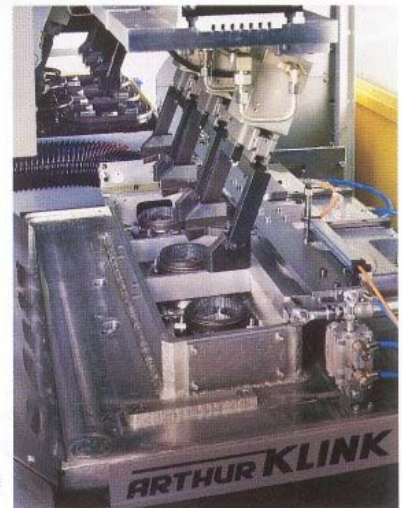
View into the working zone of a 4-station table-up hard broaching machine
