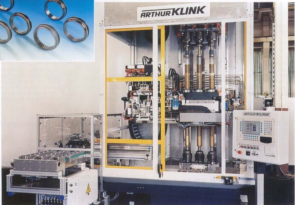
Internal table-top broaching machine, mechanically driven type RISH-M 25 x 2000 x 500 / HG with automatic loading- / unloading system for manufacturing sleeves
