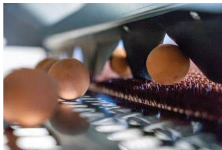
Gentle egg roll-off and extra wide plastic perforated egg belt keeps eggs clean and safe
