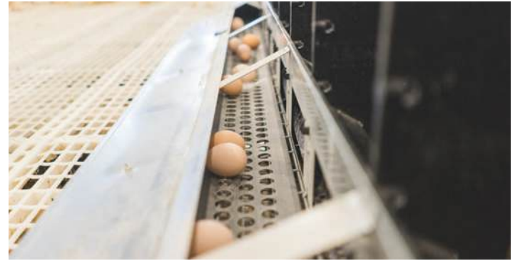
Perforated black plastic egg belt keeps eggs clean and safe. The plastic belt is easy to clean and sanitize.
