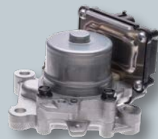
bDrive 50 oil pump housing with micro-controller
