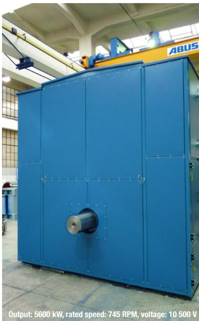
Output: 5600 kW, rated speed: 745 RPM, voltage: 10 500 V
