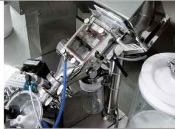
THS/PH21N-WIP: Wash-in-Place Metal Detection System.
