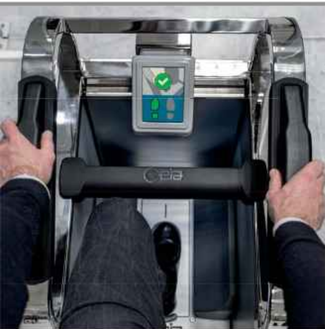
Passenger Screening with WTMD + SAMDEX and passenger body control through Explosive Trace Detector (ETD).
