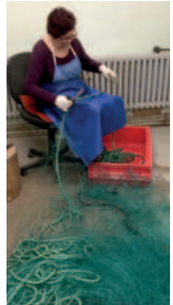
Brugte garn fraskæres. / Old lines are cut off for remounting.
