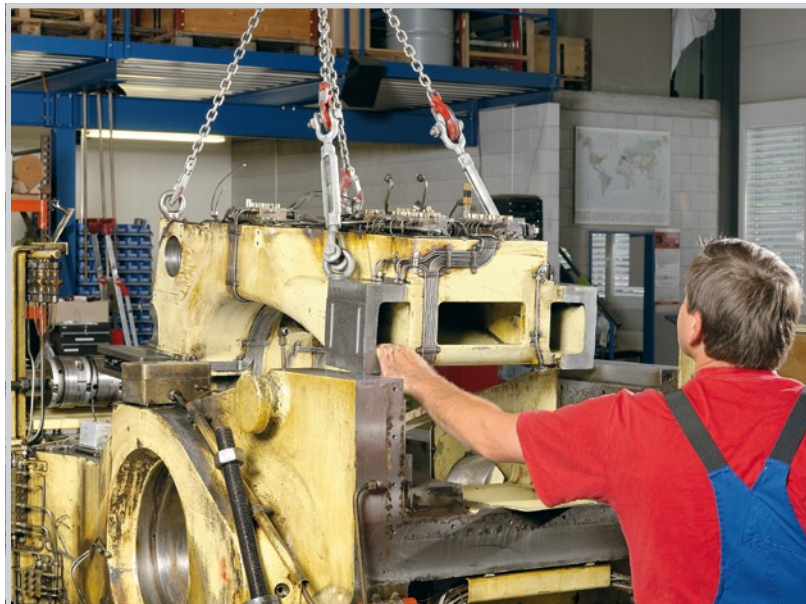
The Hatebur service engineer disassembles the machine before carrying out the rework. Here: removing the pressram from a Coldmatic AKP 4-5.
