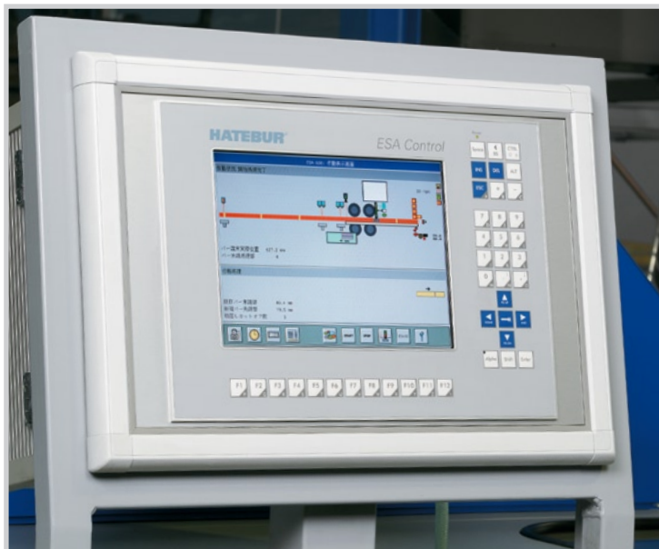
ESA 600 operating panel: from May 2010, versions with Asian and Cyrillic characters will be available.
