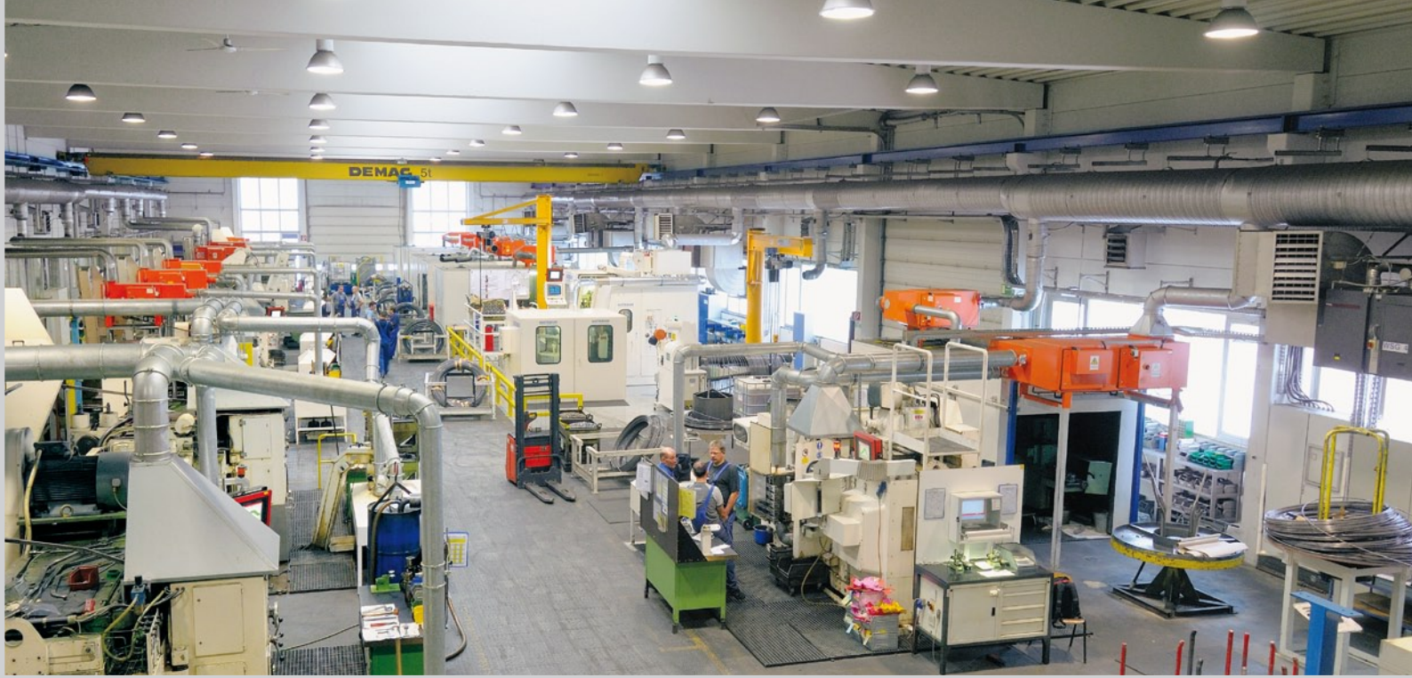
An imposing assembly of machinery with diverse coldformers. Middle right: the Hatebur Coldmatic AKP 4-5.
