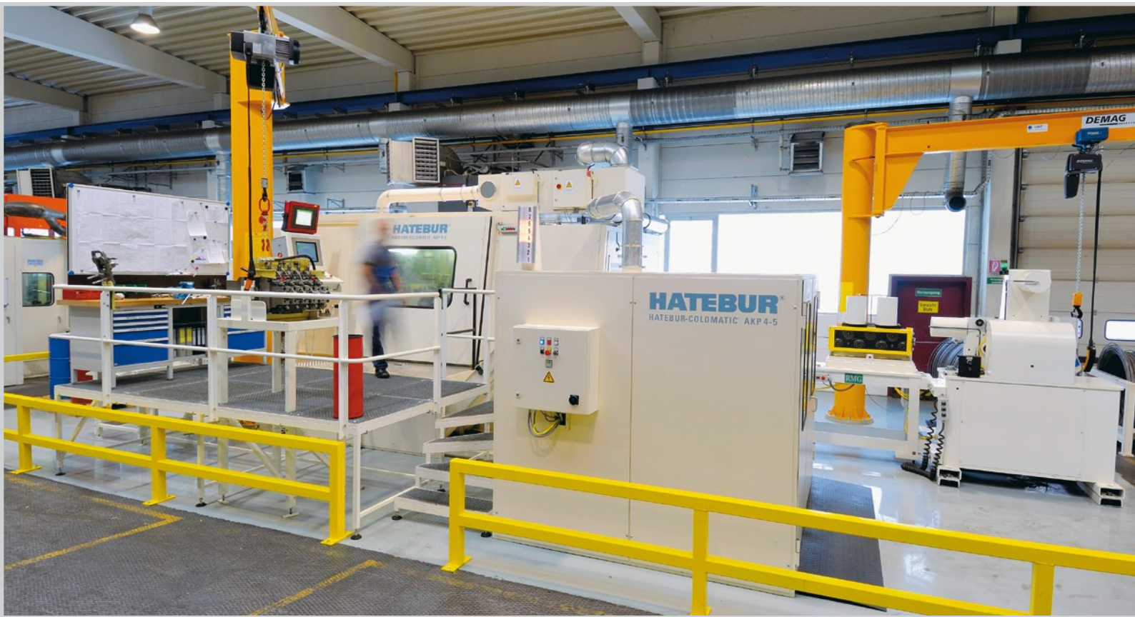
In the coldforming limelight at DURA: the new Hatebur Coldmatic AKP 4-5.
