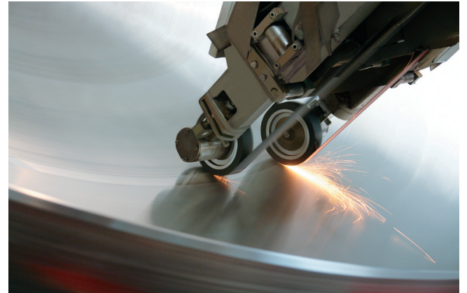
Figure 2: Surfaces can be ground to the required R_a value.
