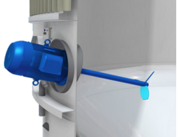
Figure 9: Agitators are installed on the side...
