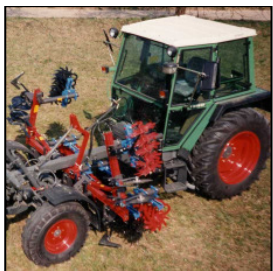
Star-Cultivator, 4-rows in the Fendt GT 275 for strawberry cultivation
