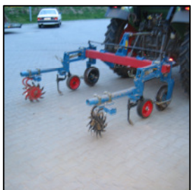
Star-Cultivator as lane-loosener
