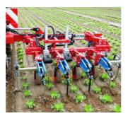
Each cylinder is controlled by the respective camera computer and moves the corresponding hoe continuously to the accurate position
