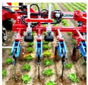
Each tool support is attached by parallelograms to the main frame.
