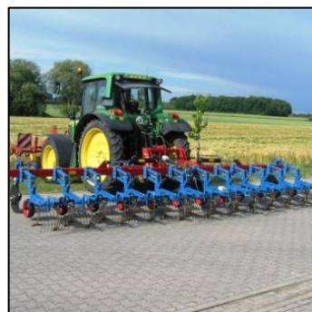
HABICHT Sugar beet Hoe, 12-rows, rear mounted with camera controlled steering
