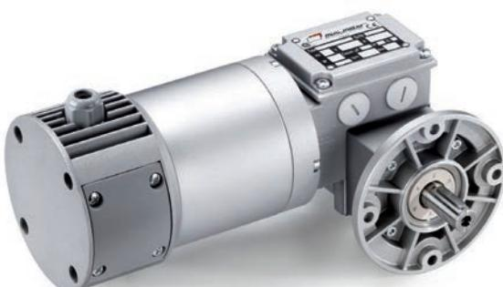
**EN/USA** Worm gearmotor with permanent magnets direct current motor, integrated with planetary reduction stage. Wheelbase 26 mm / 1.02 in.
