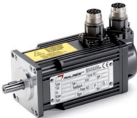
EN/USA 4-pole sinusoidal 230Vac brushless motor with resolver or encoder, totally enclosed. Rotor with NdFeB magnets. □ 35 ÷ 80 mm
