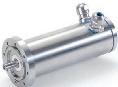
**EN/USA** Stainless steel 4-pole sinusoidal 230Vac brushless servomotor with resolver. Rotor with NdFeB magnets. Compliant to EHEDG.
