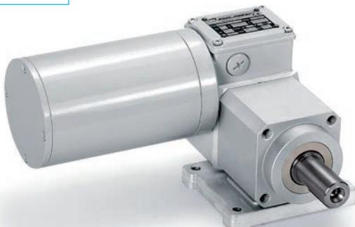
**EN/USA** Worm gearmotor with asynchronous three-phase motor, integrated with planetary reduction stage. Wheelbase 32 mm / 1.26 in.
