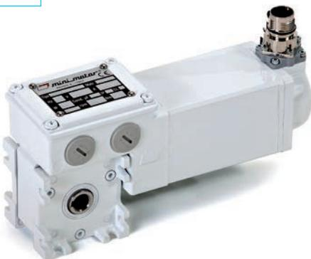
**EN/USA** Gearmotor with 4-pole sinusoidal 230Vac brushless motor, NdFeB magnets rotor, integrated with worm reduction unit.
