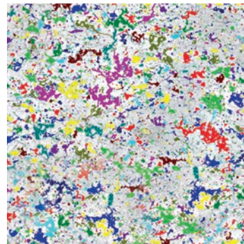
Image analysis to determine the porosity of a thermal barrier coating
