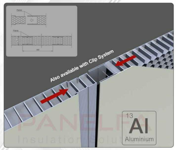
The HONEYCOMB PANEL was designed to meet the light weight requests. This product also offers an excellent finish with a single joint between panels. HONEYCOMB PANEL is a sandwich panel made of two external sheets of aluminum 0.7 mm thick, optionally coated on one or two faces with a decorative PVC layer of low flame propagation. The core is made of aluminum honeycomb, all joined by a mono component glue specially designed for this product. Available for FTG or CLIP System.
